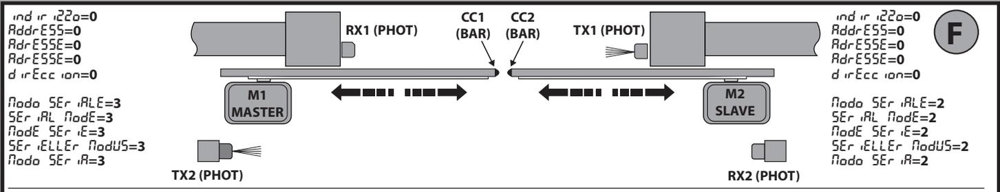
**ESEMPIO APPLICAZIONE ANTE CONTRAPPOSTE CON 2 PHOT E 2 BAR - SAMPLE APPLICATION WITH OPPOSITE LEAVES WITH 2 PHOT AND 2 BAR - EXEMPLE D'APPLICATION VANTAUX OPPOSÉS AVEC 2 PHOT ET 2 BAR - ANWENDUNGSBEISPIEL EINANDER ENTGEGENGESETZTE TORFLÜGEL MIT 2 PHOT UND 2 BAR - VOORBEELD TOEPASSING TEGENOVERGESTELDE VLEUGELS MET 2 PHOT EN 2 BAR**
